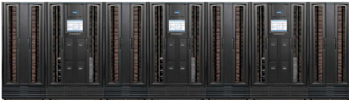
Configurations containing up to 4 LRMs and 5 MEMs store over 9,600 tapes.
