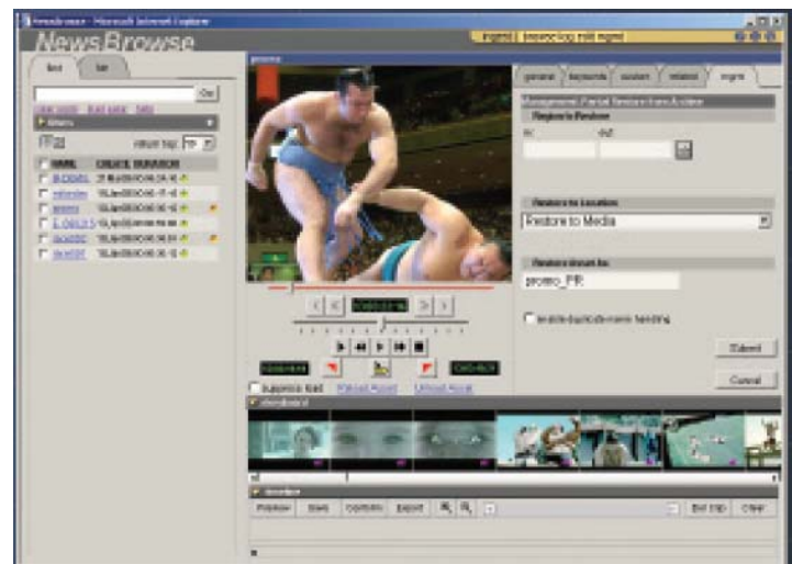
The FlashNet and Newsbrowse integration also provides Partial File Restore, allowing editors to specify in and out points to restore only a section of an archived clip
